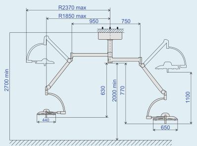
Two moveable and vertically adjustable spring arms make it possible to site the light heads in every desired position. The cardanic system (at both light heads) grants an even higher flexibility.
